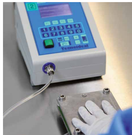
Testing pressure loss with filtered air
